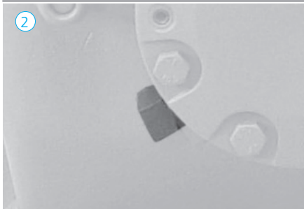
Screw-in option for oil differential pressure switch
