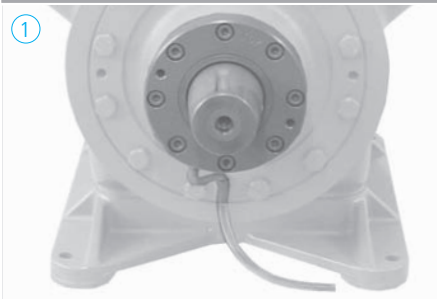
Shaft seal with piece of tube
